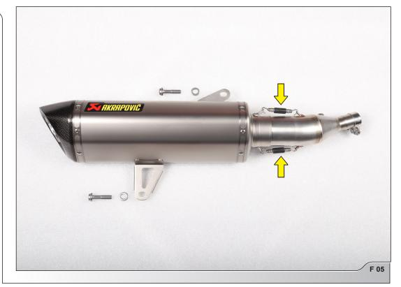
IMPORTANT: make sure, that springs pull the muffler all the way onto the link pipe – use rubber mallet if necessary to tap the connection into place!
