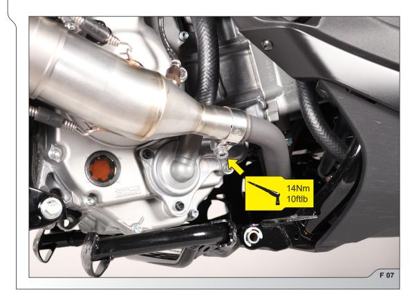
4. Tighten the marked bolt and washer from Akrapovič installation kit to the specified torque (F 08).
